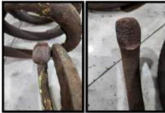
Gambar II. 7 Secondary suspension mengalami patah
